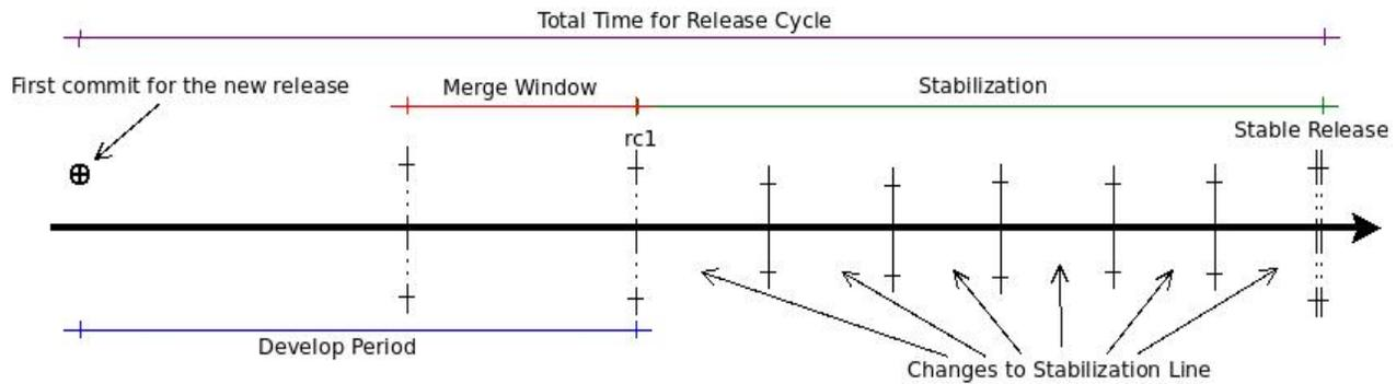
**Figure 1: Linux Release Process.** Development of subsequent releases occurs in parallel with the stabilization of a release. The two stages join during the merge window where new development is moved onto the stabilization mainline.
